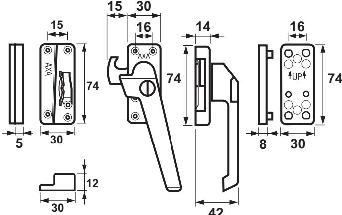
Recommended fasteners: 4,5 x 55 mm, 4,0 x 40 mm or 4,0 x 50 mm.
